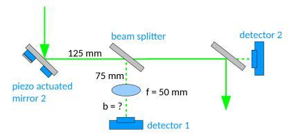
Figure 4: Setup with numerical example
