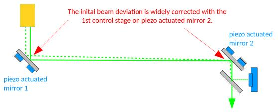
Figure 2: The principle of correcting a position error
