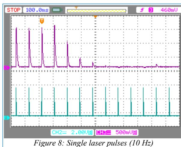
In this example only four additional pulses are required to reach the stable position. Depending on the set-up of the optical system, the pulse duration and the duration of the external trigger signal the number of required pulses can be different.
