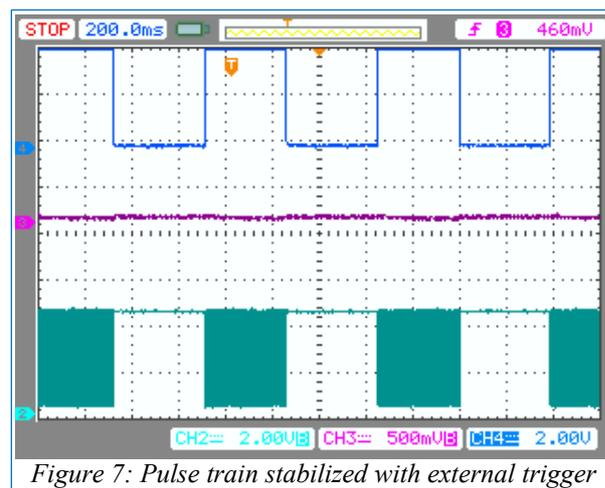
Figure 7: Pulse train stabilized with external trigger
