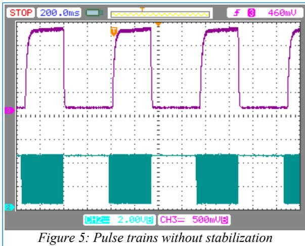
Figure 5: Pulse trains without stabilization
