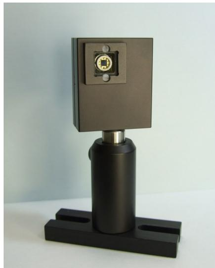
Figure 3: UV 4-quadrant diode with sensitive area of 3x3 mm<sup>2</sup>
