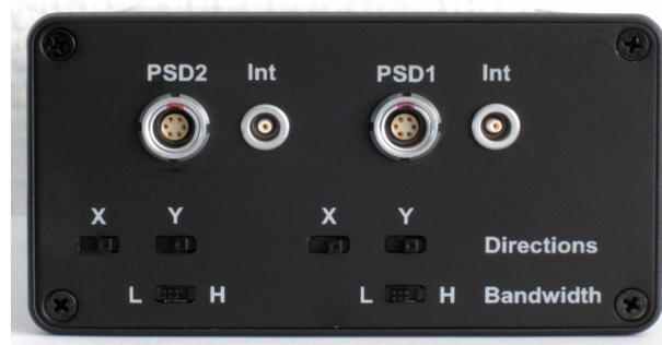
Figure 2: Right panel with PSD input connectors and intensity output connectors
