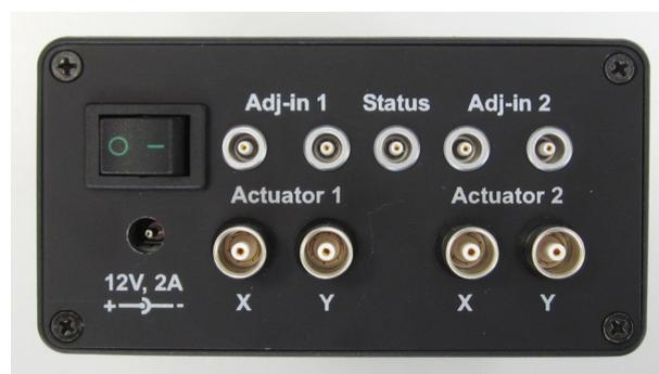
Figure 1: Left panel with four additional “*Adj-in*” inputs for x and y position of two PSDs
