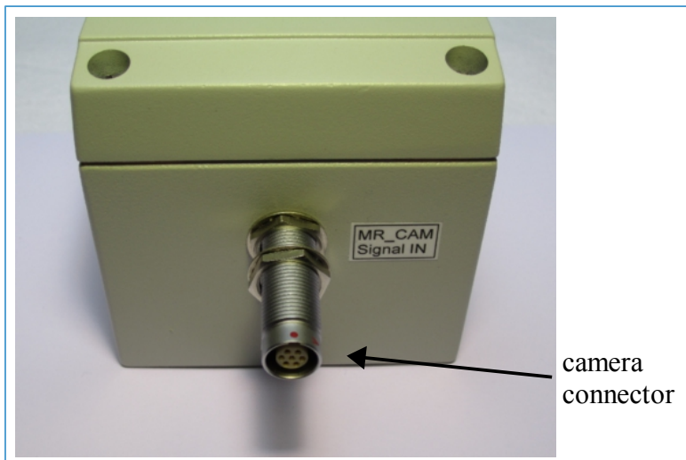
Figure 2: Filter box (front side)
