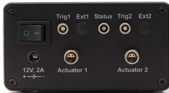
Figure 16: Left panel of control box with trigger inputs
