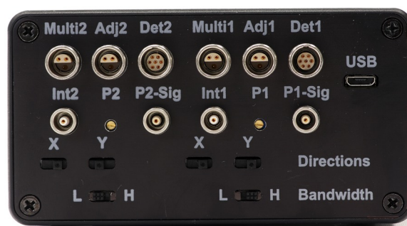
Figure 24: Right panel with additional “Adjust-in” inputs for x and y position of two PSDs
