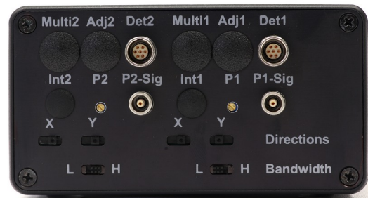
Figure 7: Input connectors, P factor adjustment and switches on right side
