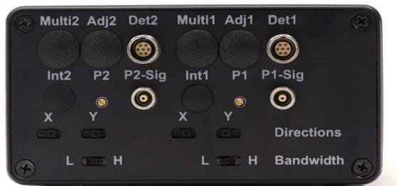
Figure 2: Input connections, P factor adjustment and switches on the right side
