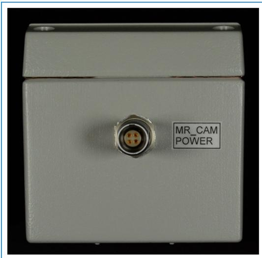
*Figure 4: Filter box (front side) with connector for power cable*
