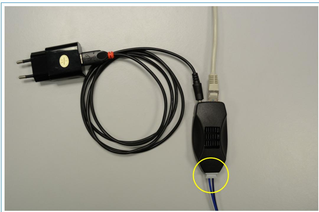
*Figure 8: Fibre connection at converter*
